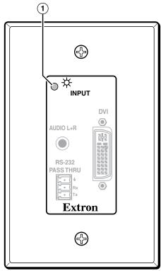
**DVI 201 A D Tx Transmitter Front Panel**
